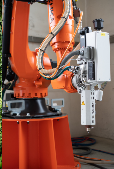
source: Hans Weber Maschinenfabrik GmbH, Weber DXR system for 3D printing with pellets
